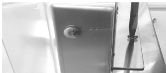
Screw the safety (back of cover)
