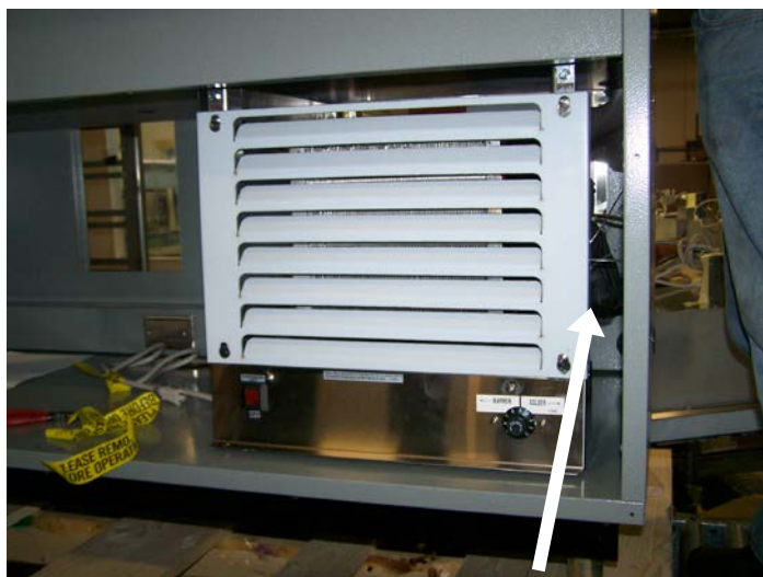
4) Remove lower shelf and louver. Pull condensing unit out so AXV can be held during adjustment. AXV is located here.
