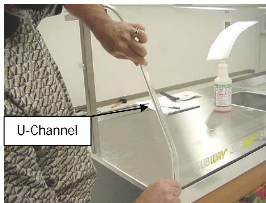
Step 10. Put clear vinyl U-Channel over each end of the curved glass. If vinyl channels do not seat properly, apply NSF
