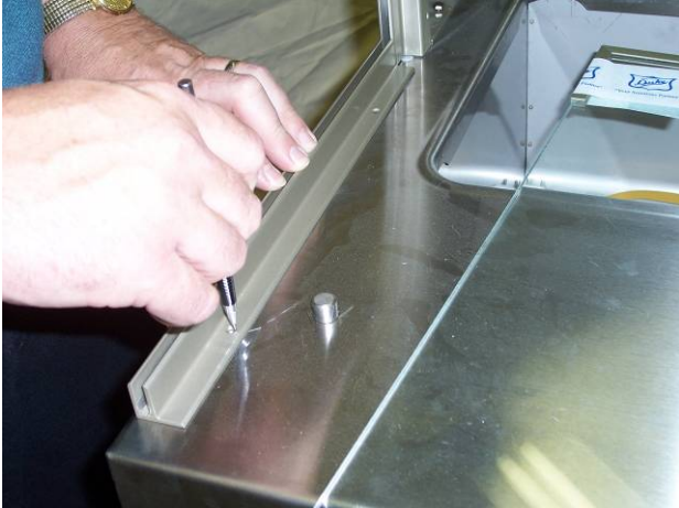
26) Mark the two holes and set the horizontal channel aside.
