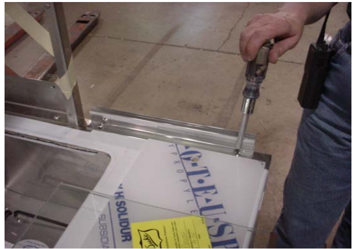
Line up the holes in the extrusion with the holes on the outside end of the Hot Food unit.
