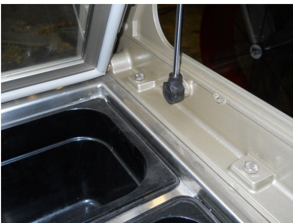
29) Reattach bolts, pylons, and glass clips
