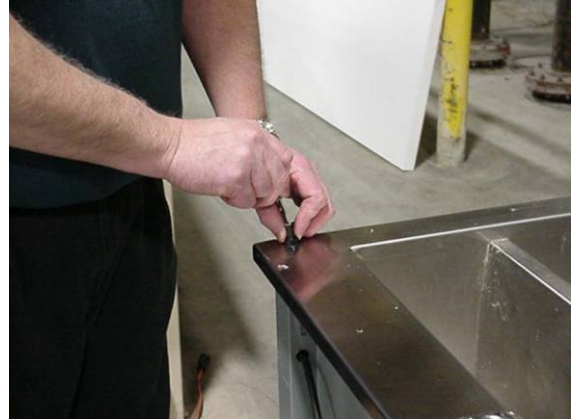
14) Slide a Grommet over Wire and snap into drilled hole.
