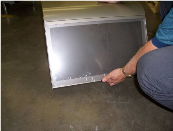
7) Remove the frosted and clear plexiglass from the new Day Cover by pulling out then pulling down from the bottom. Set these aside.
