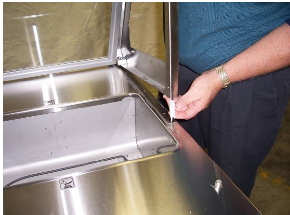
4) Lift cover slightly and unplug electrical connection.
