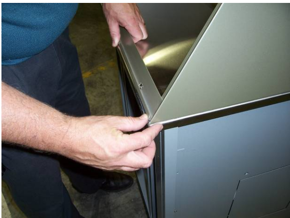
8) Set the new Day Cover on unit. Line the front and sides of Cover flush.
