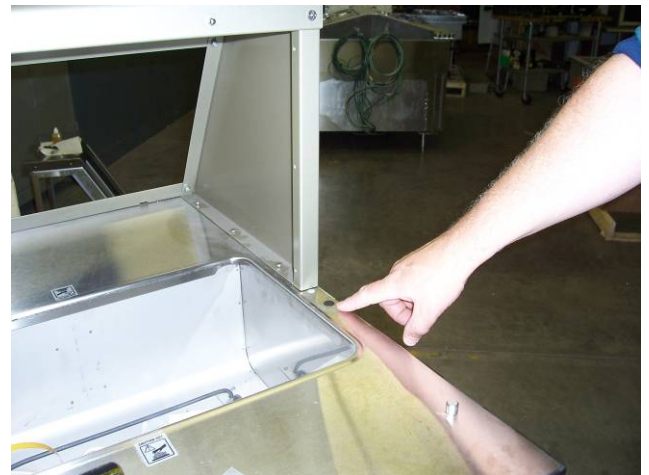
31) Plug the two holes on opposite side on unit.
