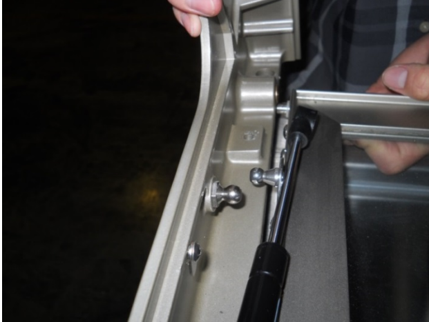
13) Pull pylon from glass pin
