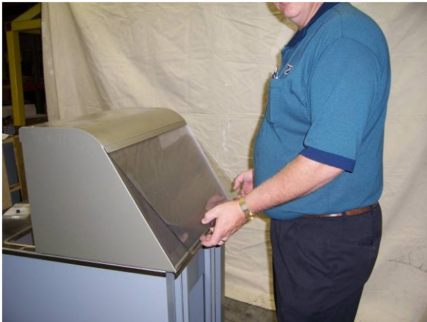
34) Place clear plexiglass into place by sliding in at top, pushing in bottom and dropping into channel.
