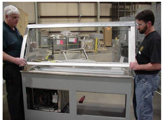
17) Place new day cover on top of unit. Caution: Make sure pylons do not spread apart and allow glass door hinge pins to come out of hinge holes.
