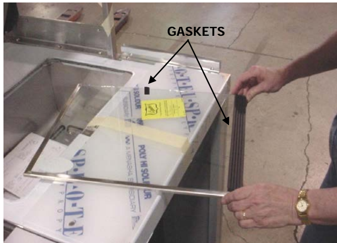
Place gasket on to lower edge of glass and small gasket on unprotected edge of inside glass.
