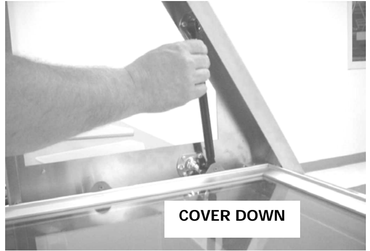
Reinstall the dampening cylinder by pressing it on to the ball joint connector.
