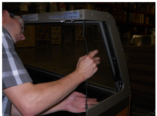
30) Slide the right end glass (if needed) in and tighten the end glass clips
