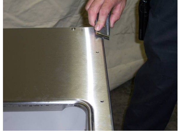
6) Use a razor blade to remove any remaining silicone.
