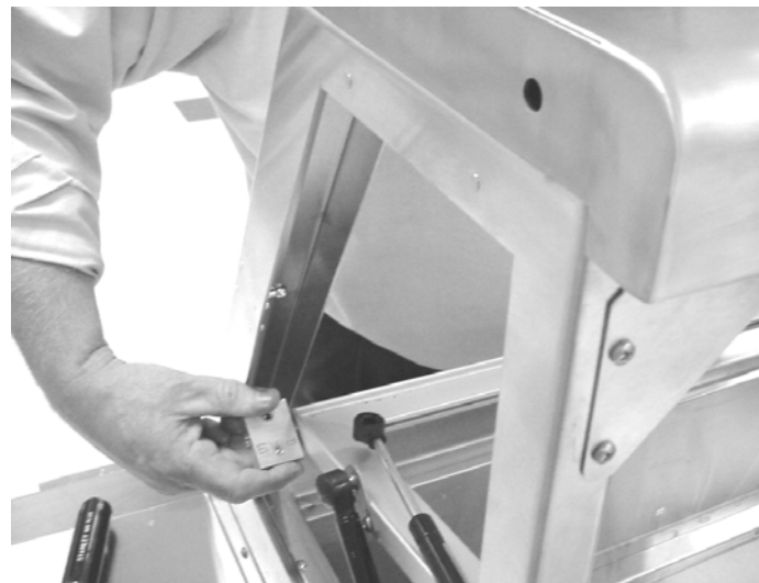
Carefully lift the day cover from the front and the back raising one side higher than the other, tilting it so that the hinge block can work its way to where the end glass piece opening is. Remove the hinge block and continue lifting and maneuvering the day cover until it is clear of the unit.
