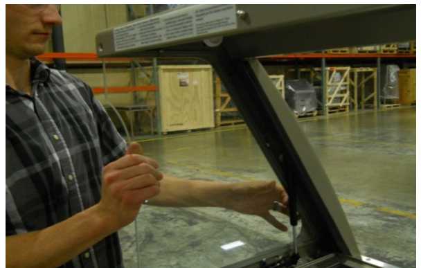
18) Slide the left end glass (if needed) in and tighten the end glass clips
