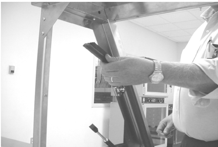
Remove rubber gasket from the Day Cover pylon.
