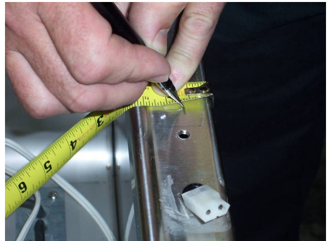
13) Measure and mark the location for a new hole to run the electric for the lights. Measure \frac{1}{2} " back from line which marks the back edge of the pylon log. Measure \frac{5}{8} " in from the ledge of the top. Use a center punch to mark this location.
