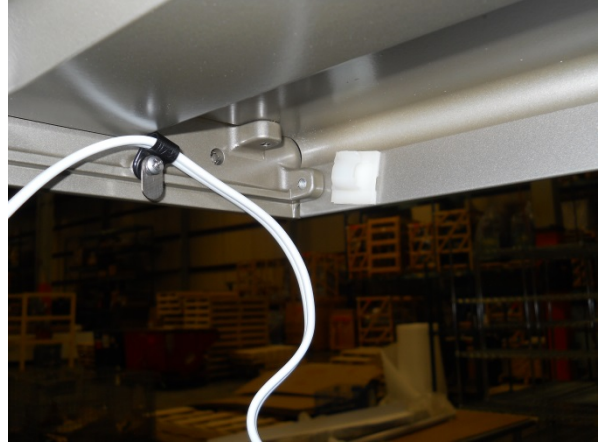
26) Reattach cord retaining clip and screw
