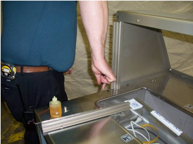
28) Tap holes; making sure to use oil on the tap.
