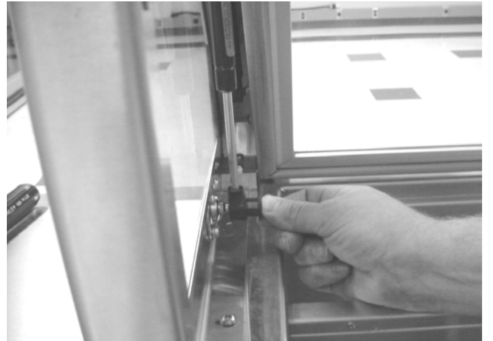
Reinstall ALL End Cap Locks on all four cylinders.
