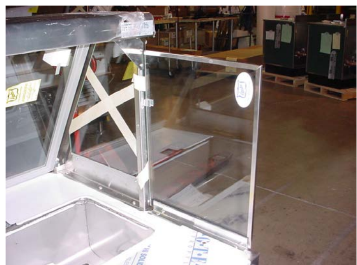
Hot Food with End Glass installed.
