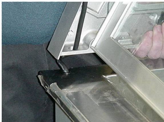
18) Feed light wire up through hole in end pylon.
