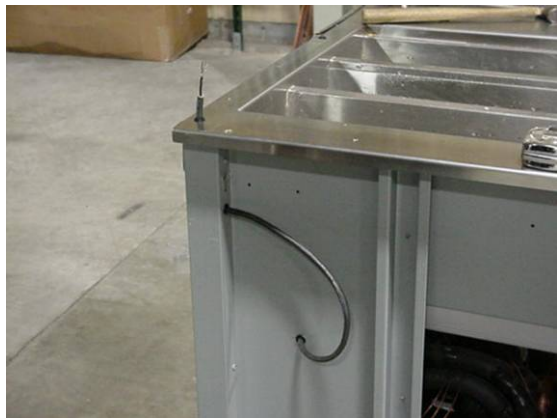
15) This wire routing will keep wires from interfering with Front Décor Panels.
