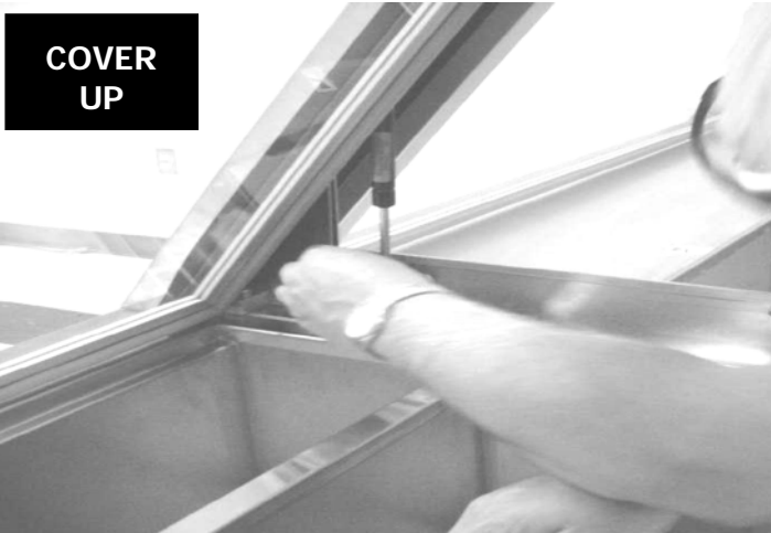
Lift the cover to open position for installing the power gas cylinder.
