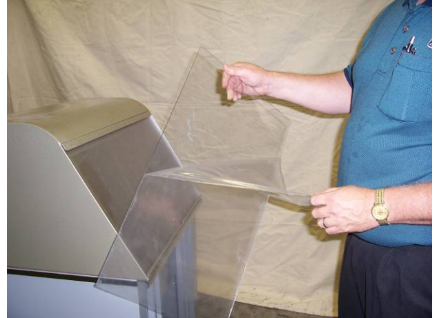
33) Peel plastic off clear plexiglass before installing.
