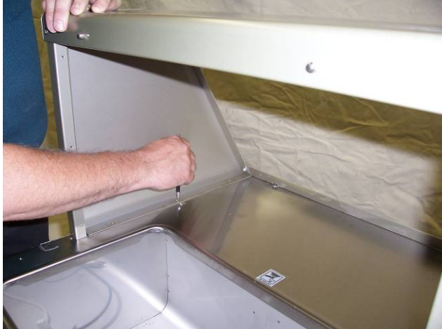
10) Mark the 6 holes to be drilled.
