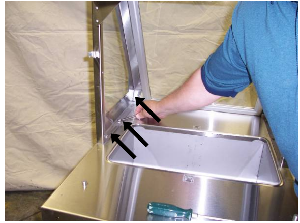
2) Remove the 3 bolts from each end pylon that secure Day Guard to unit.
