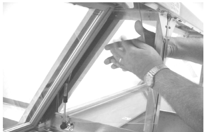
Reinstall the end glass by screwing on the bottom glass angle holder, inserting the end glass and screwing on the top angle piece.
