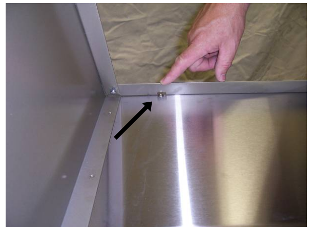
9) It may be necessary to remove one of the front screws if it does not align with the notch in the lower front rail.
