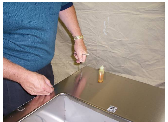
15) Using a 10/24 tap, tap each of the 6 holes. NOTE: Be sure to use oil on your tap.
