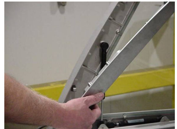
16) Remove front filler from side of the pylon that has the light wires. Keep filler for re-attachment later.
