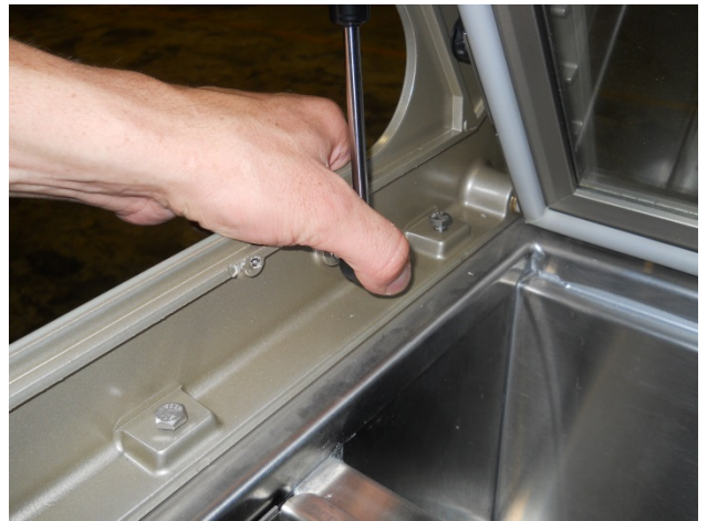
16) Reattach shocks to new pylon, note that the glass will need to be raised to get other end on
