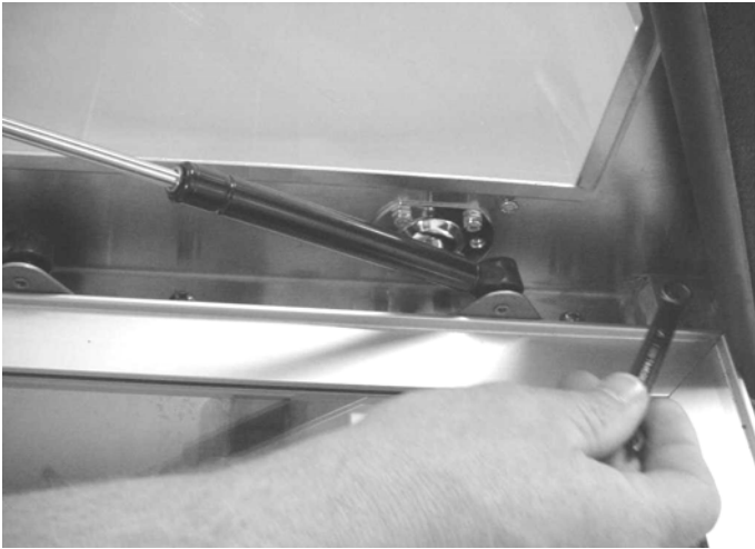
Use the 3/8" wrench to tighten nuts on the hinge mounting block on both sides.
