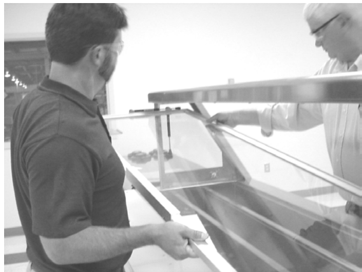
Carefully lift the day cover from the front and the back raising one side higher than the other, tilting it so that the hinge block can work its way to where the end glass piece opening is. Remove the hinge block and continue lifting and maneuvering the day cover until it is clear of the unit.
