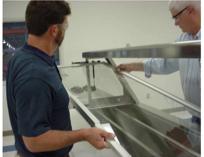
4) Carefully lift the day cover from both sides as shown. Raise one end higher than the other, tilt enough so that the hinge block can work its way to the end glass opening. Remove the hinge block and maneuver day cover until clear of the unit.
