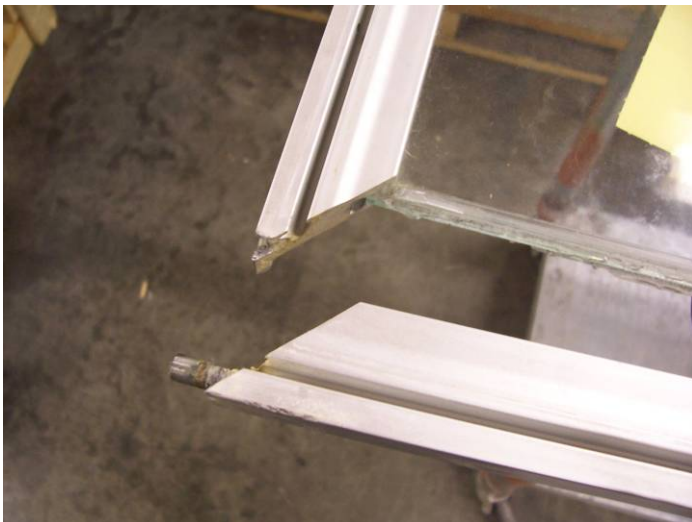
5a) Once removed, inspect. Depending on the level of damage to the day cover, clamping may be required. (See Fig. 5b)
