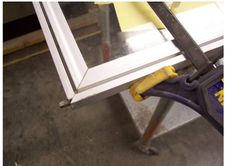
5b) Use a 24" or larger clamp to close the corner.
