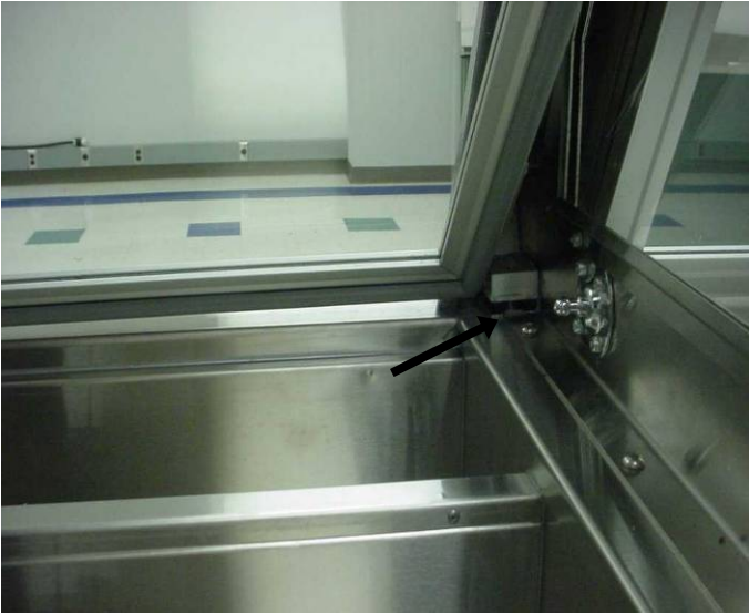
3b) Pry the hinge block with a screw driver to loosen it.
