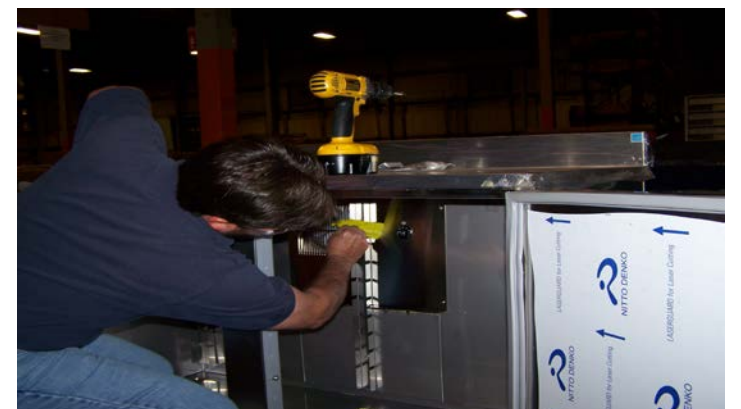
If tightened, loosen the two screws holding the center rack channel in place.
