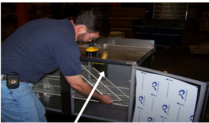
Unplug power cord from rear of unit. Allow interior of unit to come to room temperature. Wipe any moisture from Fan Cover. Remove the wire racks and place aside.
