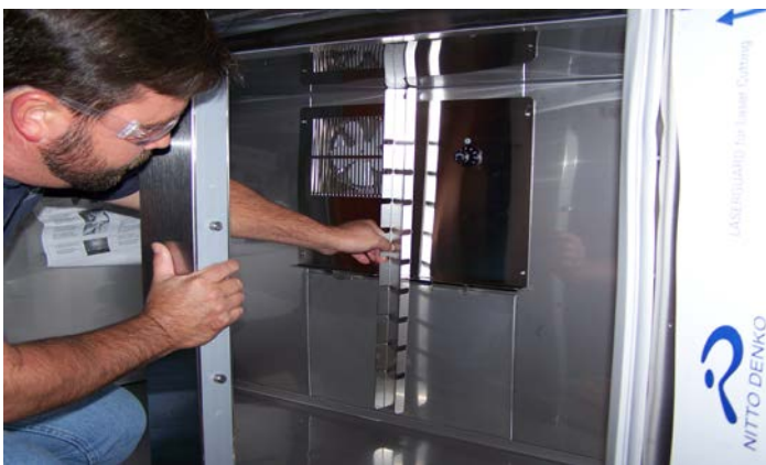
Remove the center rack channel by lifting up and sliding the keyholes over the screw heads. Set aside.
