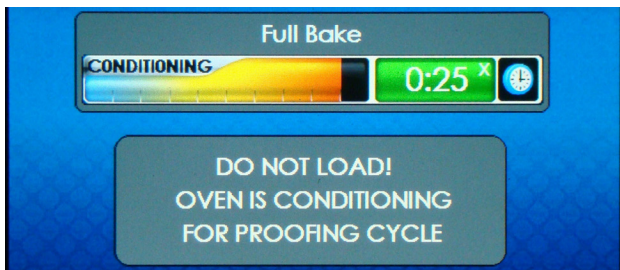
Figure: Recipe Conditioning Screen (if oven is not conditioned for proof and bake recipe; i.e. Full Bake):
