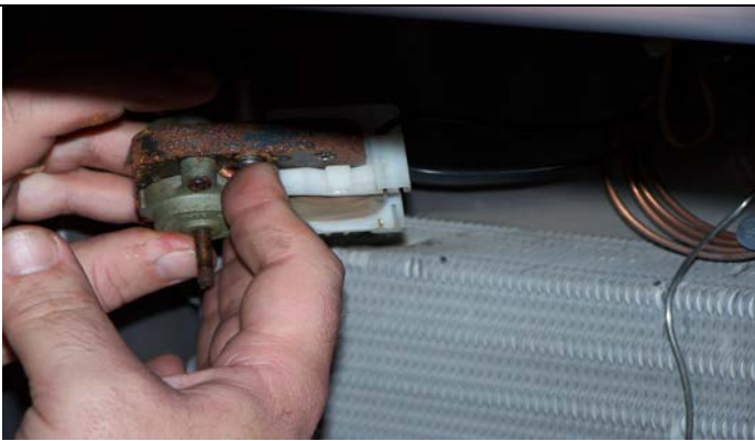
Place the (2) #6 SS Internal Tooth Washers over the screws and re-tighten the screws holding the fan motor to the unit. (If existing screws are damaged in any way, use the (2) new ones provided.) Re-install the fan blade over shaft of the motor.
