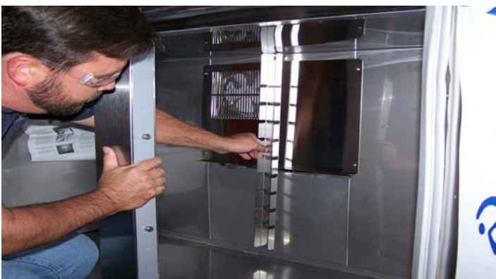
Re-Install the center rack channel support by sliding the keyhole slot over the screws in the rear liner. (These may be tightened to eliminate any vibration noise.)
