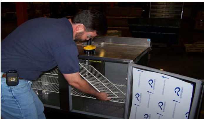
Unplug the power cord from the wall outlet. Remove the wire racks and place aside.
