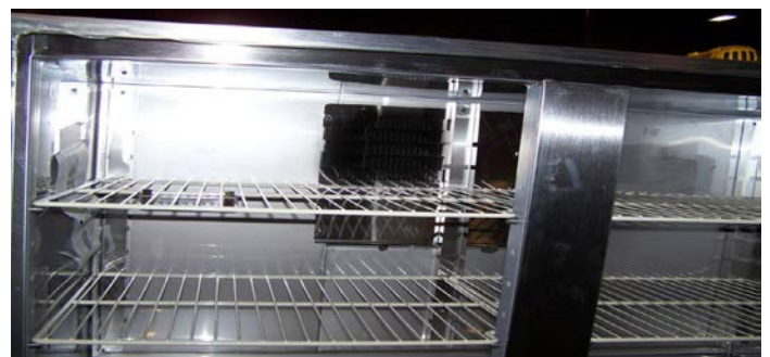
Reinstall the four wire racks. Plug the unit back into the power supply. You are now ready for use once the cabinet pulls back down to the proper temperature (between 33 and 41 degrees F).
