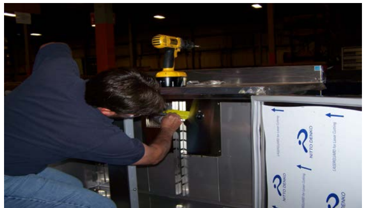
If tightened, loosen the two screws holding the center rack channel in place.
