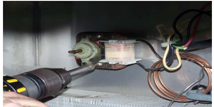
Unscrew the (2) existing " screws holding the fan motor in place. (If these screws are not damaged, they may be re-used.) Be careful not to allow the fan motor to fall and damage the blade or shaft.
