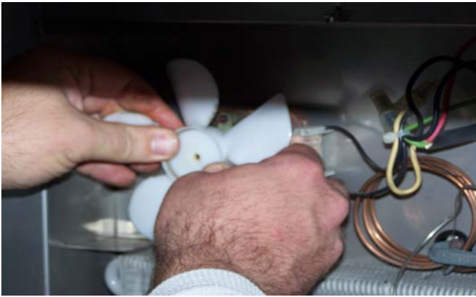
Remove Fan Motor Blade to get to the two mounting screws.
