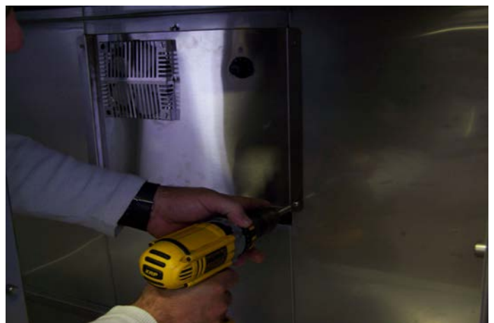
Unscrew the (4) screws holding the Fan Cover in place and remove from the unit. Now, the Fan Motor should be exposed to you.
