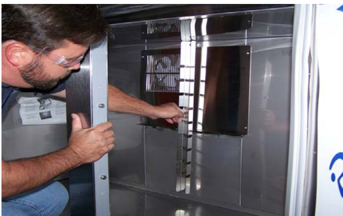
Remove the center rack channel by lifting up and sliding the keyholes over the screw heads. Set aside.
