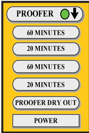
Figure 29: Proofer Controls Screen
