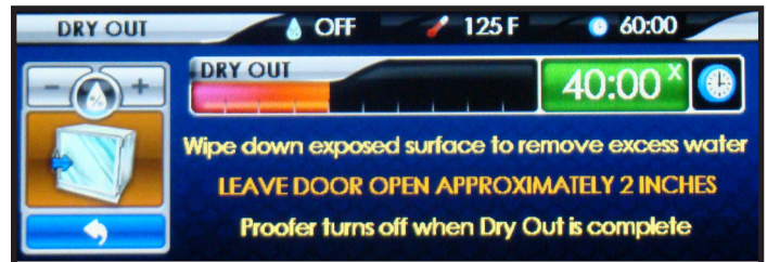
Figure: Proofer DRY OUT Screen
