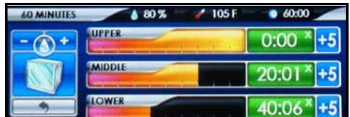
Figure: Proofer Complete Alarm Screen
