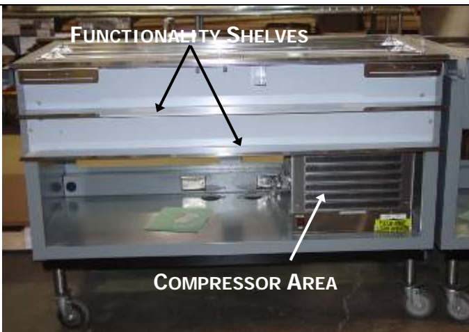
This is the operator's side of the Tri-Channel Unit.
