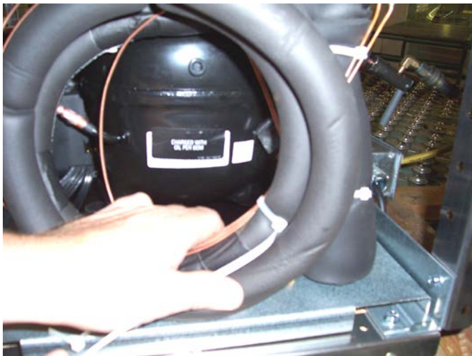
21. In the three o'clock position, take care not to secure the capillary to the last coil of the courtesy loop to avoid binding when sliding the compressor out for service.
