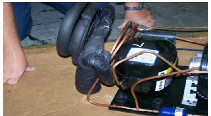
13. Begin reassembly by placing the liquid line courtesy loop in between the suction line and the accumulator as shown.
