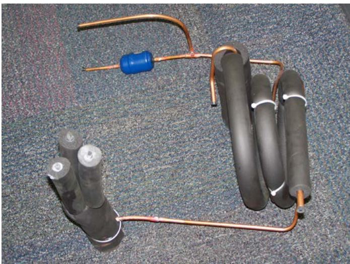
12. The new liquid line assembly has a 3 circuit Automatic Expansion Valve and an Accumulator (under the insulation). It also contains a Filter Drier . (uninsulated)
