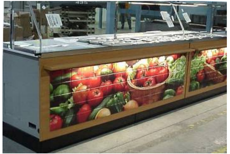
To remove the décor panel from a unit with stationary glass, loosen the screws in the glass extrusion and pull up on the panel, slide it from the lip.
