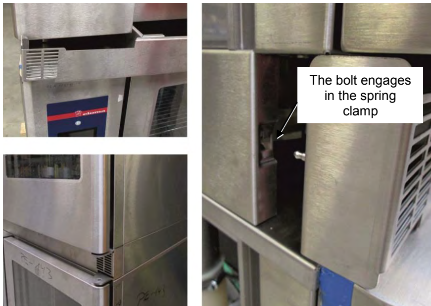
Fig. 60: Installation of the front foot panelling
