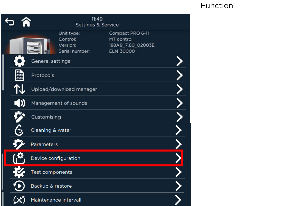
Figure 64: access device configuration
