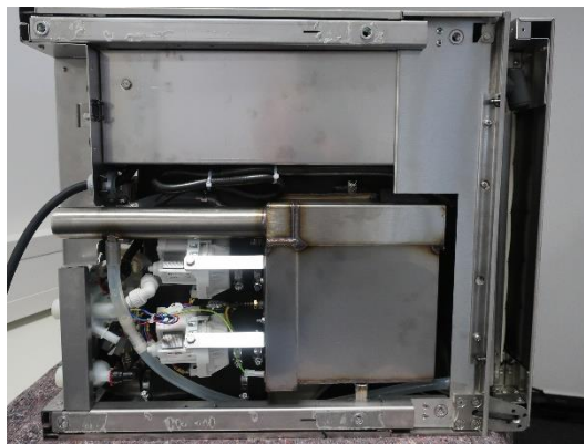
Figure 51: autoclean box and pumps
