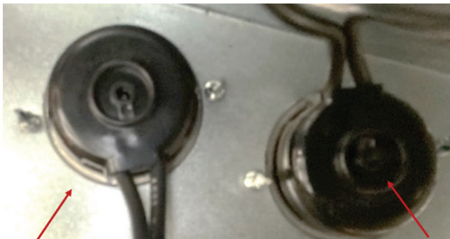
Primary Auto-Reset Thermal Limit Switch Manual Secondary Limit Switch
