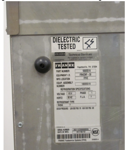
The HCMF Unit Serial Number is located below the Model Number & Data sticker, which is on the back of unit.
