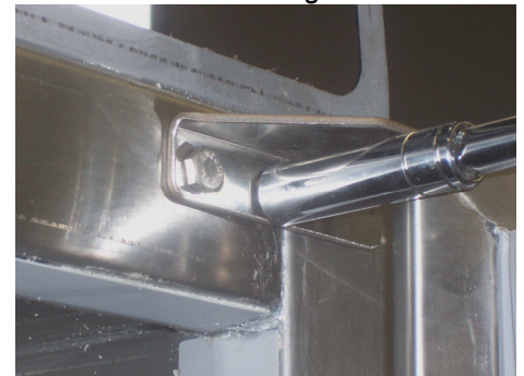
Mount lower hinge, place door on bottom hinge pin & secure top hinge.
