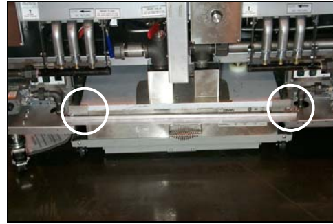
Figure 1. Retainer latches securing filter pan.
