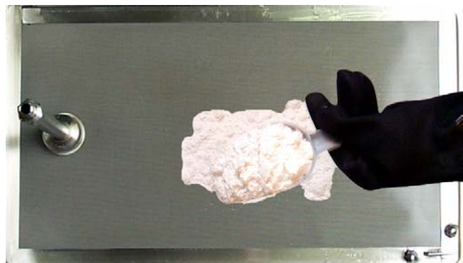
Applying filter powder to screen.
