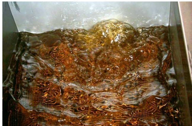
Allow the oil to bubble for 15-30 seconds after the filter pan is empty to clear the oil-return lines.
