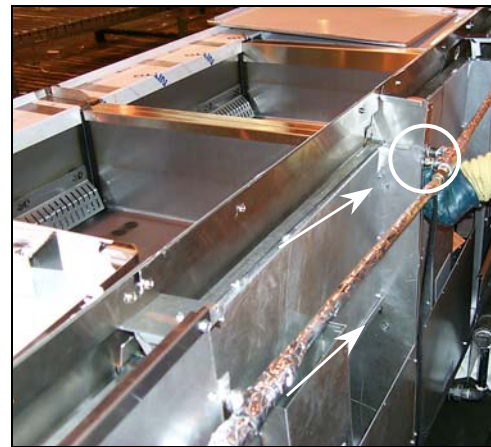
Figure 5. Rear cabinet connection holes. Note oil return line fittings.
