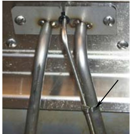
Secure probe bulb to the element back in two places with metal wire wrap (arrow).
