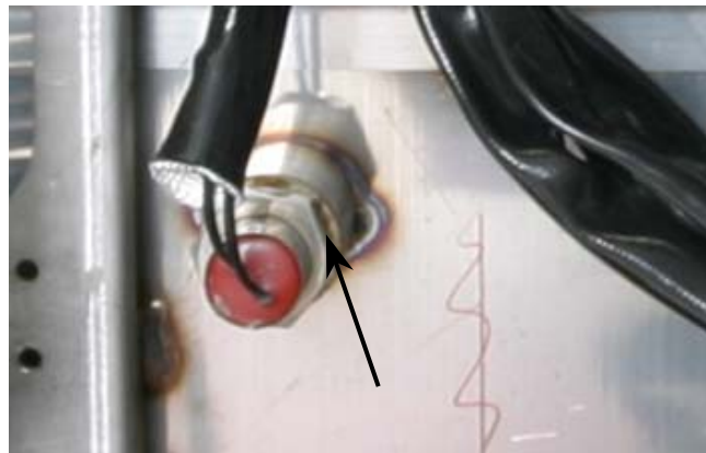
Place wrench here when removing and installing high-limit.
