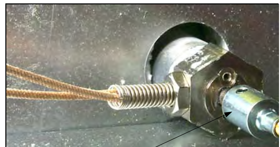
On G-Model fryers, the shaft connecting the exterior thermostat knob to the frypot-mounted thermostat must be disconnected.
