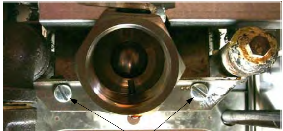
Step 5: These screws on each side of the drain valve must be removed to lower the burner from the frypot.
