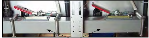
Step 2: On FM35 fryers, sections of the drain system must be removed to access the burner assembly.
