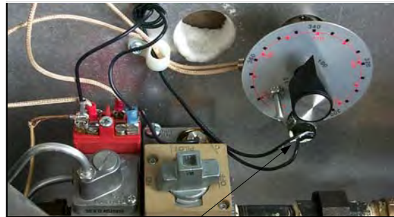
The high-limit thermostat on the standard MJ35 is located below the thermostat dial.
