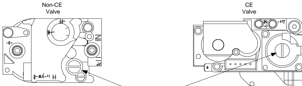
GAS VALVE REGULATOR CAP
