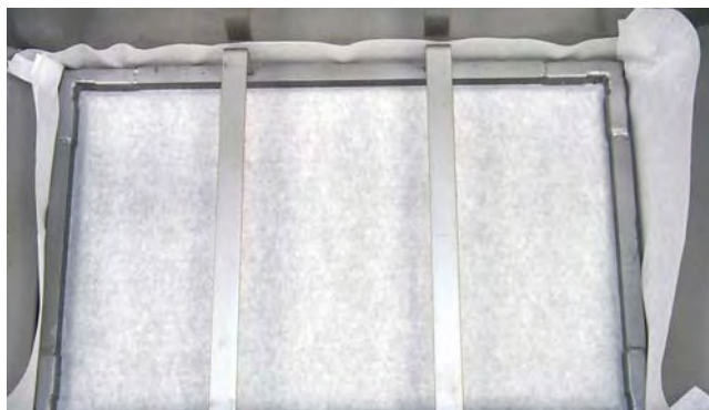
Hold-down ring positioned correctly over filter paper in filter pan.
