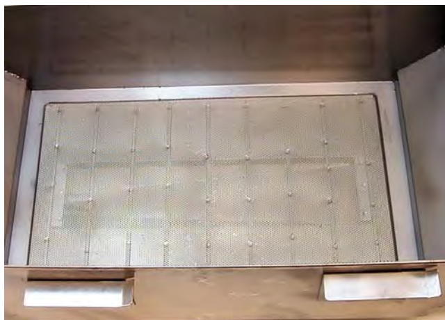
Support grid properly placed in filter pan.
