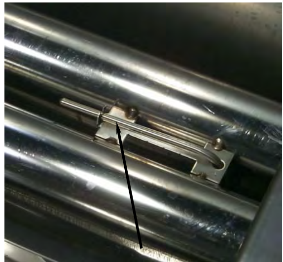
Electronic thermostat probe in frypot (arrow).
