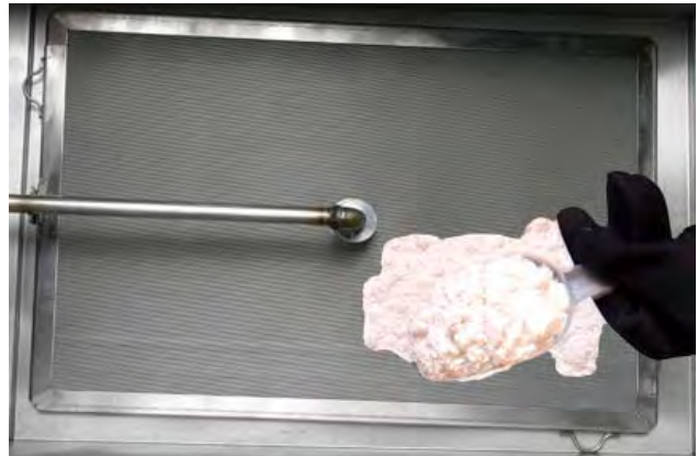
Applying filter powder to filter-leaf.
