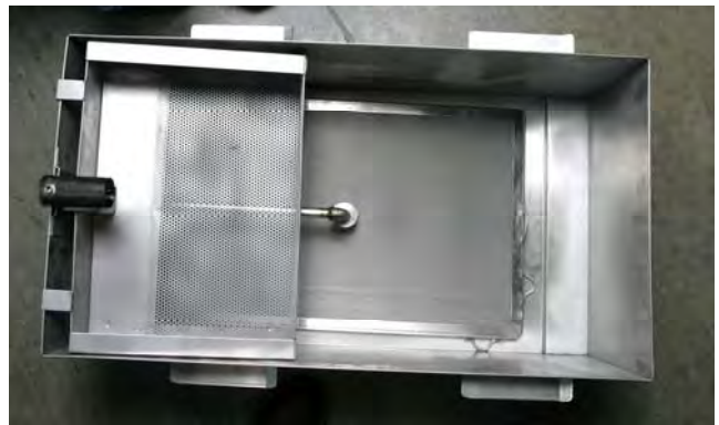
Crumb screen properly placed in filter pan.
