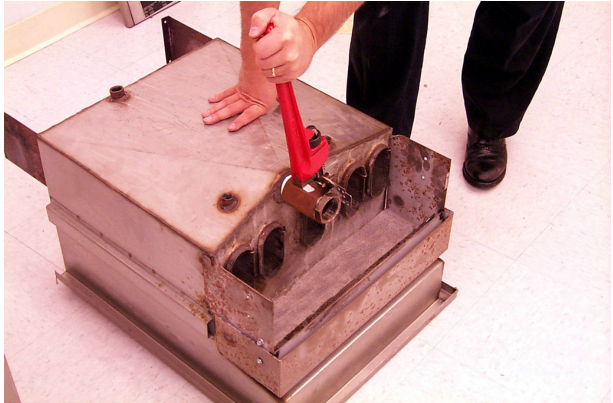
Removing drain valve from frypot.
