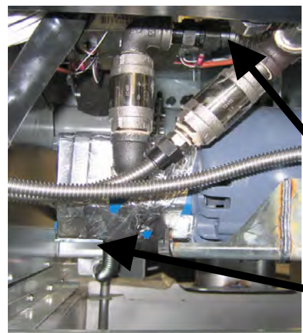
Disconnect flexlines indicated by the arrows.
