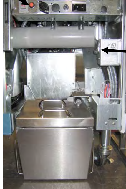
Melting unit power switch
