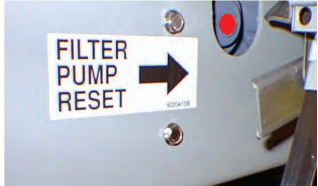
Reset switch location: Old-style FP111
