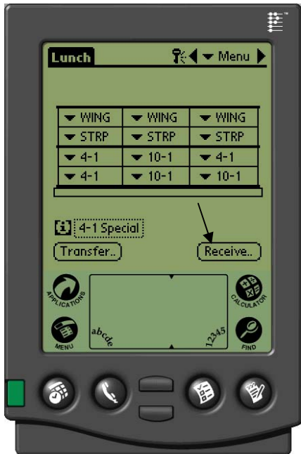
Figure 1: To prepare the Palm Pilot to receive data from the HCP cabinet, tap the receive button.
