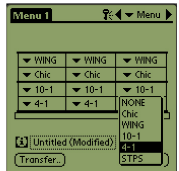
Figure 4: Cabinet configurations are built on the screen of the Palm by first choosing a Menu and then selecting a slot for each item, which are chosen with the pull-down at each slot position.
