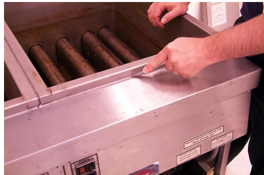
Cutting frypot seal prior to frypot removal.
