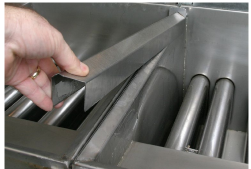
Removing the joiner strip.
