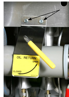
Oil-return handle bracket and screws.
