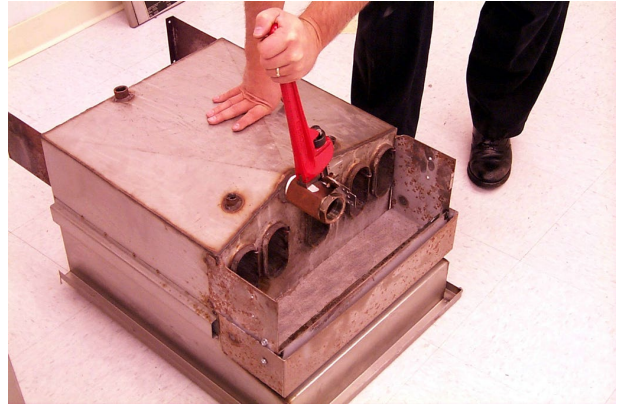
Removing drain valve from frypot.
