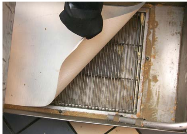
Placing new sheet of filter paper over paper support screen.
