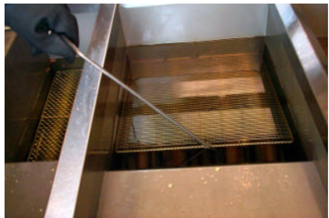
Replace drop-in grid/crumb screen as oil level rises. Use an appropriate tool (fryer cleanout tool, etc.) to place the screen in hot, filtered oil/shortening.
