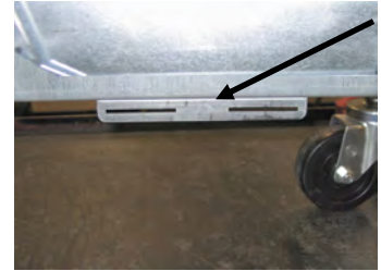
Figure 1: Attach alignment bracket to bottom of ATO box brace.
