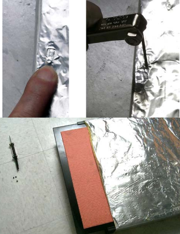
Figure 13: The heater plate slides from the insulation.
