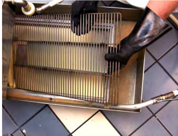
Removing paper support screen from pan.
