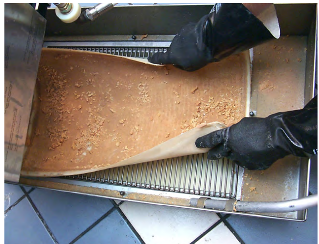
Removing dirty filter paper from pan.
