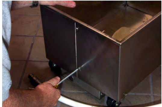
Remove screws securing outer panels.
