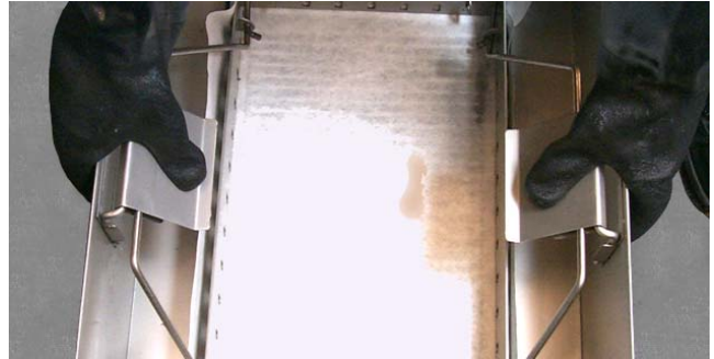
Locking hold-down ring in place.
