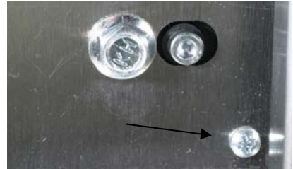
Fig. 9 Loosen the hex bolt and remove the allen screw (arrows, upper photo). Some row positions may have an additional screw securing the bezel to the cabinet (lower photo). Push through the access port (arrow, upper photo), if necessary, to remove the bezel from the cabinet .
