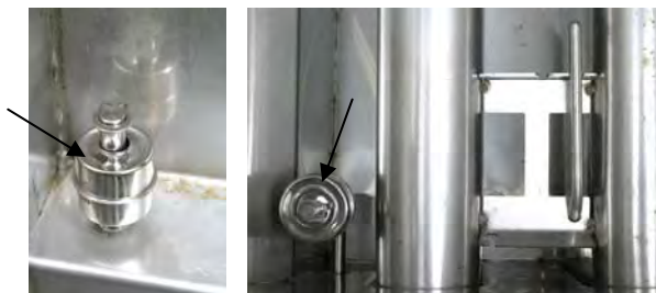
Figure 1: The float switches (above and right) should be cleaned periodically to eliminate starch buildup, which can impede the motion of the floats. Take care, however, to ensure the shafts are not dislocated or the movement of the float hindered.
