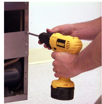
Removing gas manifold shield.
