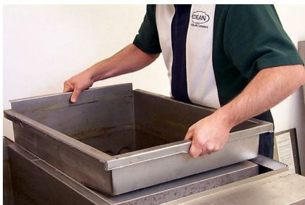
Lift cookpot from rethermalizer.
