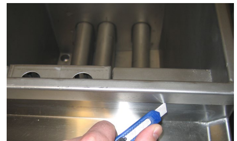
Cut cookpot seal prior to cookpot removal.
