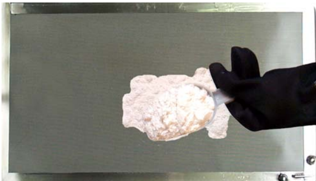
Applying filter powder to screen.
