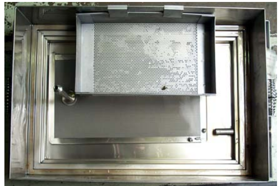
Placing the crumb screen.
