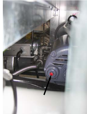
Filter pump reset button, accessed from the front of the fryer.
