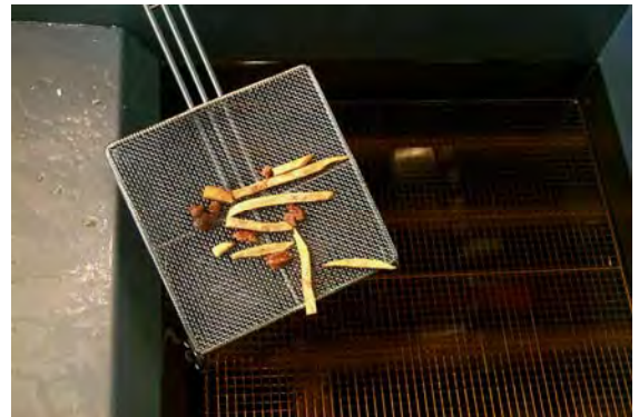
Prior to filtering, skim any large debris from oil in frypot.
