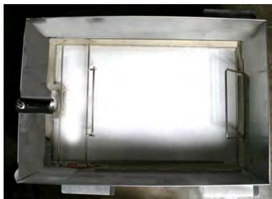
The hold-down ring is shown resting on the filter pad. The notches in both are turned toward the pick-up tube.
