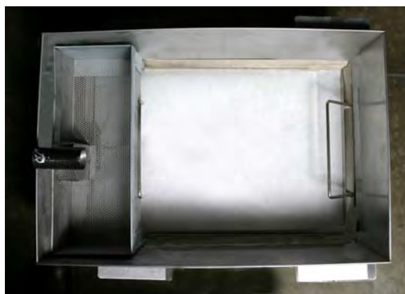
The filter pan is shown with the pad, hold-down ring and crumb tray in place.
