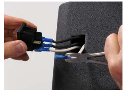
Remove harness connections from four switch terminals.
