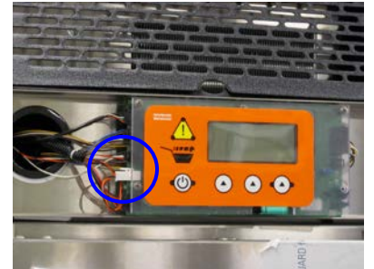
Disconnect 24-volt power lead at Main Control Board [24v].
