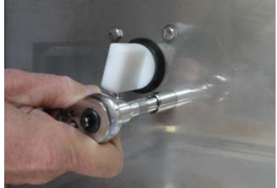
Remove and discard the four block mounting bolts.
