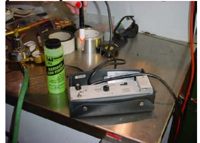
If system pressure is too low or the leaks difficult to pinpoint, pressurize system with 150 PSIG [10.5 Bar] of Nitrogen and use an electronic leak detector or soap solution.
