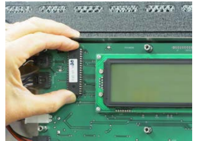
[Photo 7] When installing chip
