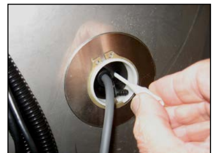
After removing the small plastic plug, use a 2 mm [1/16"] screwdriver to adjust sensitivity.
