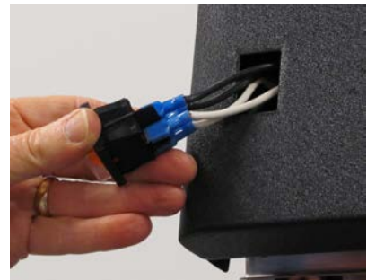
Pull switch out to access terminals.
