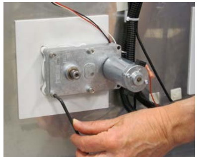
Remove the four motor mounting screws.
