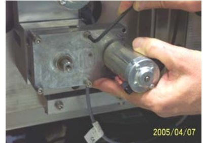
Remove the four motor mounting screws.
