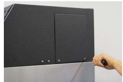
Remove the right side service access panel.
