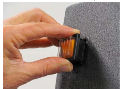
Push in new switch until locking tabs engage & bezel is flush.
