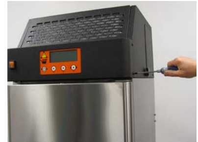
Remove four front control panel cover/bezel screws.
