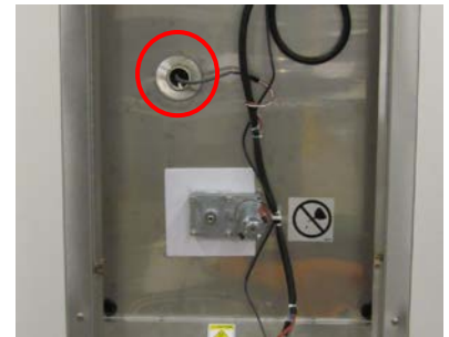
A low product sensor is just left-of-center above rotor motor.
