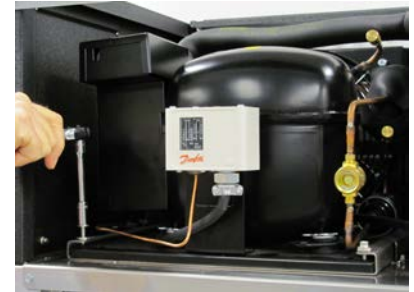
Loosen the four Condenser Assembly base retaining screws.
