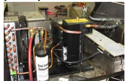
Add a few ounces of R-404A refrigerant & pressurize to 150 PSIG [10.5 Bars] with nitrogen.
