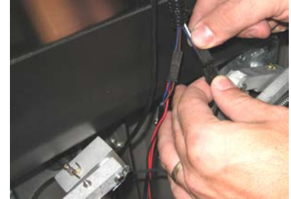
Disconnect sensor lead from Main Wiring Harness.
