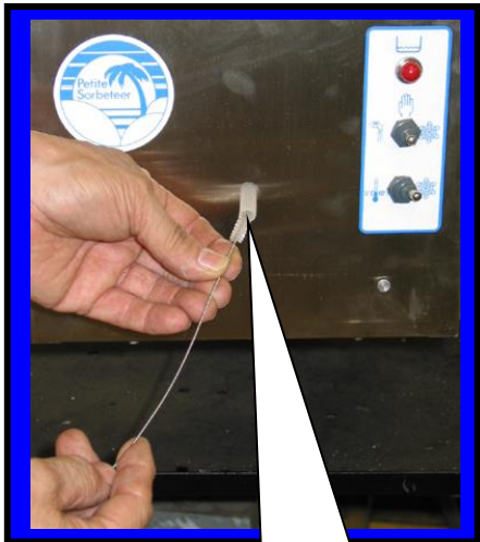
Insert long brush F6526 into drip tube
