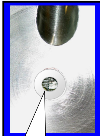
Push brush all the way in until it can be seen behind the ceramic ring
