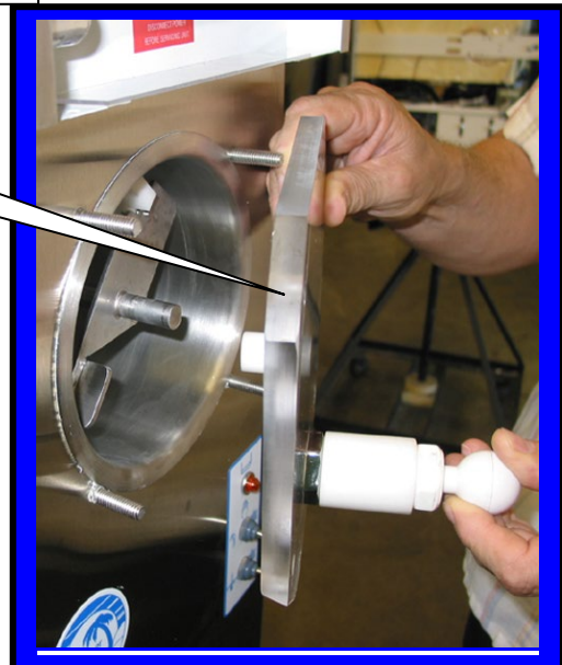
Installing faceplate C6521 onto front of Machine.
