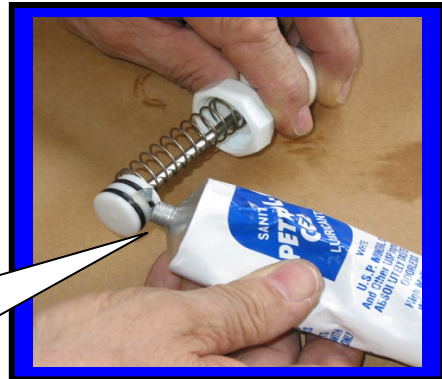
Installing O-rings onto plunger F 0491
