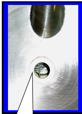
Push brush all the way in until it can be seen behind the ceramic ring
