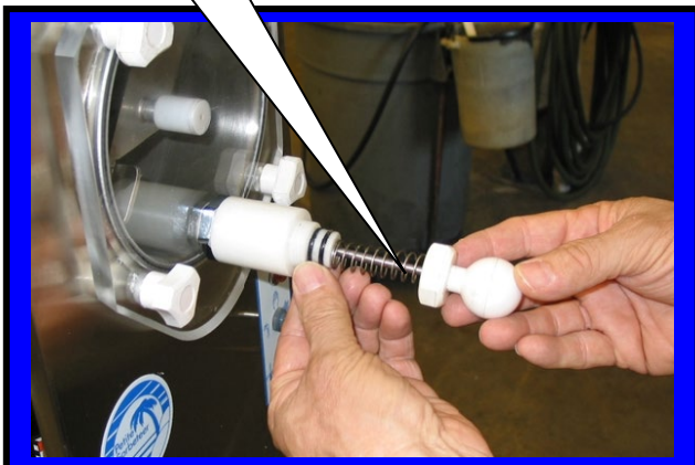
Installing faceplate C6521 onto front of Machine.
