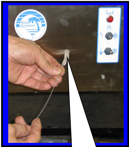
Insert long brush F6526 into drip tube
