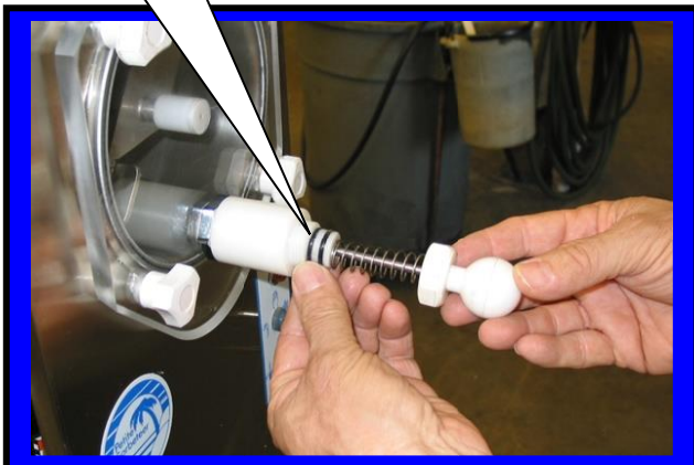
Installing Plunger assembly C6513P into faucet body
