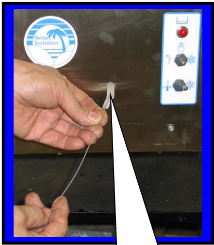
Insert long brush F6526 into drip tube
