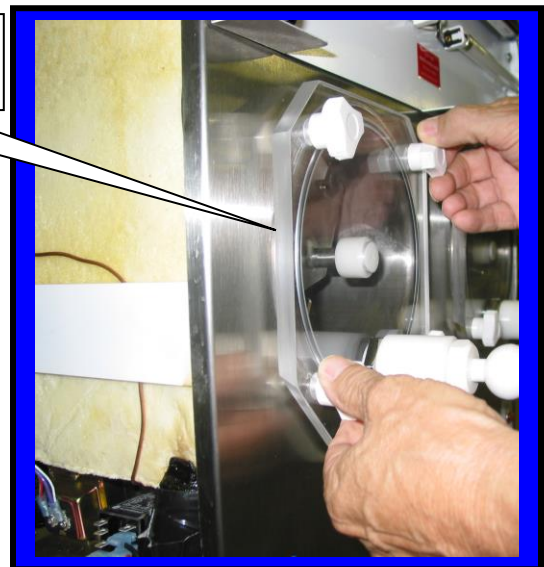
Installing faceplate C6521 onto front of Machine.
