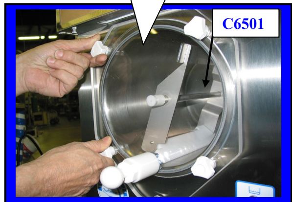
Installing large Faceplate onto front of Machine.
