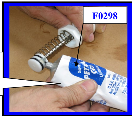
Lubricating O-rings with Petro-Gel
