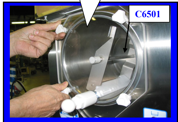
Installing large Faceplate onto front of Machine.
