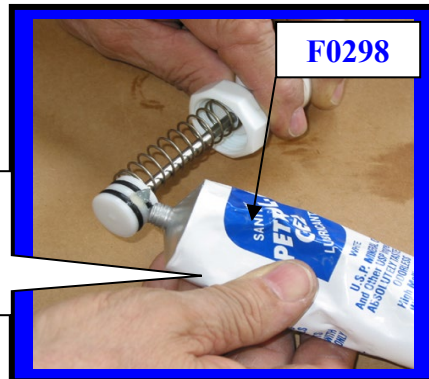
Lubricating O-rings with Petro-Gel
