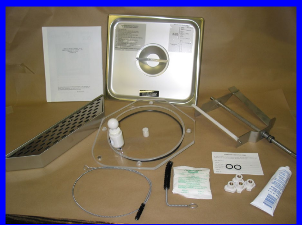
Beater Bar, Drip Tray, Faceplate, Faceplate Knobs, Hopper Cover, Petro-Gel, Sanitizer, Spare Faucet O-Rings, Wire Brush, Water Hoses & Manual.
