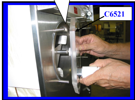
Installing Faceplate onto front of Machine.
