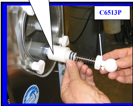
Installing Plunger Assembly into Faucet body
