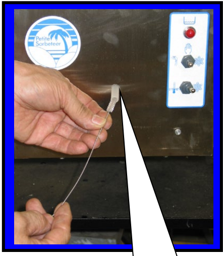
Insert long brush F6526 into drip tube
