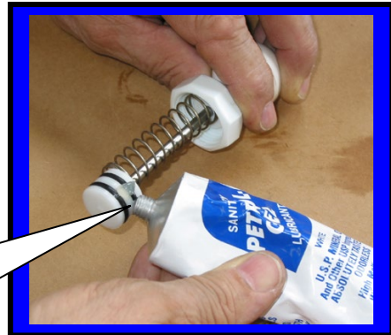
Installing O-rings onto plunger F 0491
