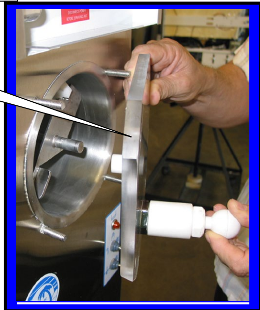
Installing faceplate C6521 onto front of Machine.
