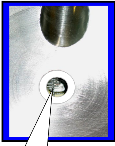
Push brush all the way in until it can be seen in the middle of the ceramic ring
