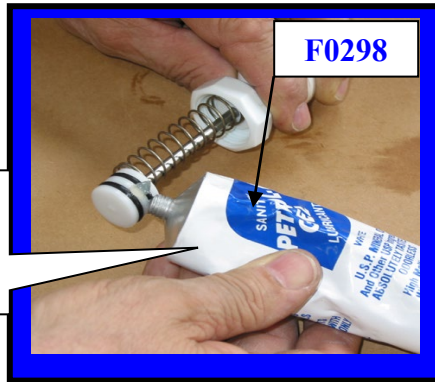
Lubricating O-rings with Petro-Gel
