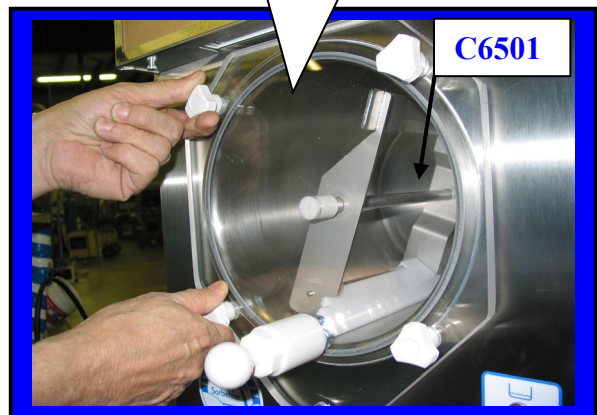
Installing large Faceplate onto front of Machine.
